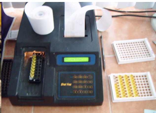
Figure 20 Measure of Acetylcholinesterase Activity in the Spectrophotometer
